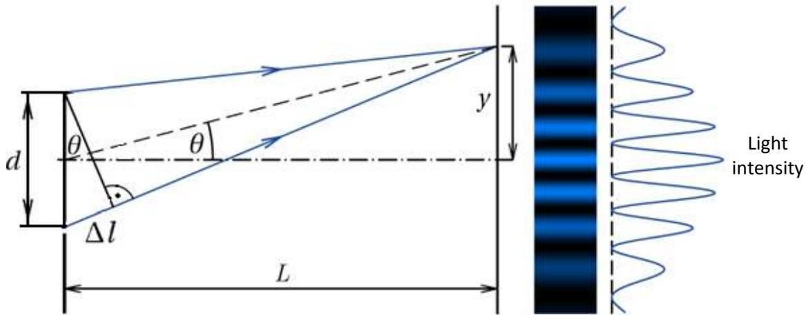
**Fig. B2** Diffraction of light on an obstacle.
