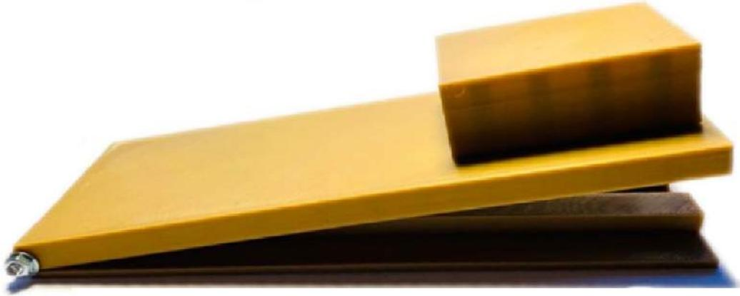
**Fig. B5** Inclined plane apparatus.
