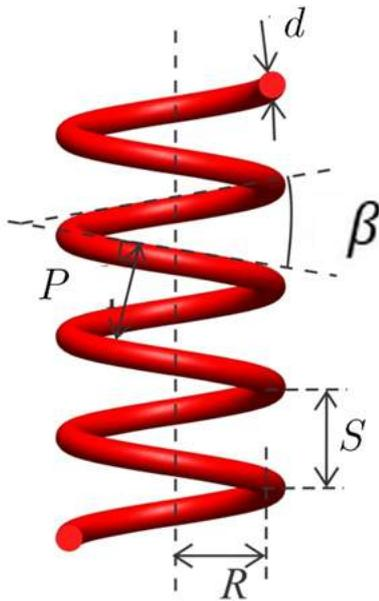
**Fig. B3a** Geometry of the helical spring.
