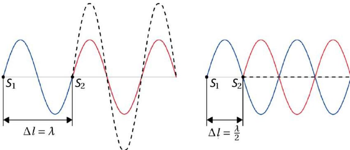
**Fig. B1** Constructive and destructive interference.
