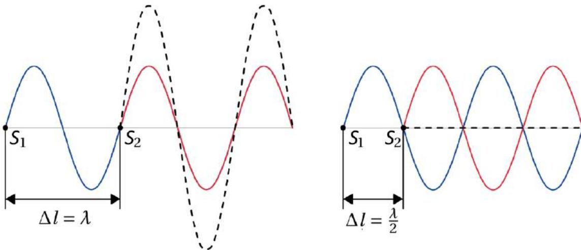
**Fig. B1** Constructive and destructive interference.
